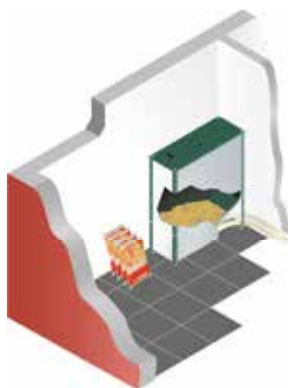
Pellet box 350 litre with suction head manually filliable
